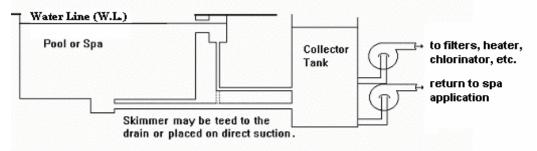
Conceptual Gravity Drainage System – Direct Suction Removed from the Pool Currently there are no voluntary standards for gravity drainage systems or collector tank specifications.
