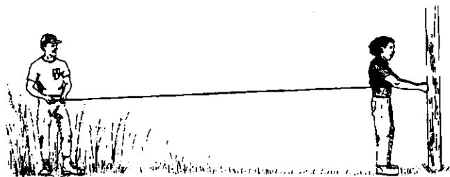
Measuring from benchmark to locate the on-site wastewater system.
