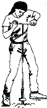
Making soil boring with a hand auger.
