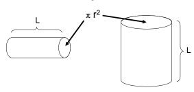
• Operating volume (ft³) of a cylindrical pump tank:
