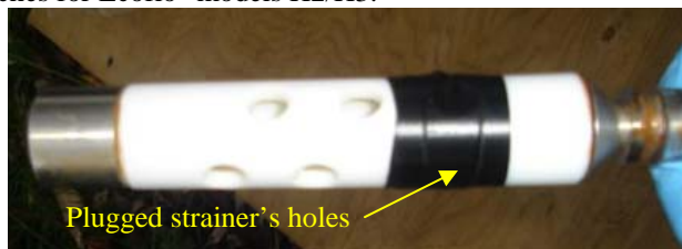
Figure 1 Strainer of the suction line
