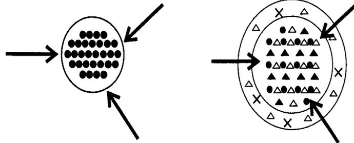
1. Water enters a granule of water-soluble monocalcium phosphate —  $\text{Ca}(\text{H}_2\text{PO}_4)_2 \cdot \text{H}_2\text{O}$ .
