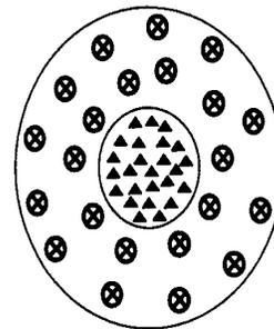
4. The iron (Fe), aluminum (Al), or manganese (Mn) react with the phosphate to form insoluble compounds. This reaction ties up the phosphorus, making it inaccessible to plants and further movement in the soil.
