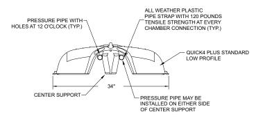
**12.** If installing multiple rows of chambers, follow Steps 1-9 to lay the next row of chambers parallel to the first. Keep a minimum separation distance between each row of chambers as required by local code.
