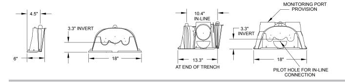
Quick4 Plus LP High Flow Splash Plate (not to scale) Required when pumping into system
