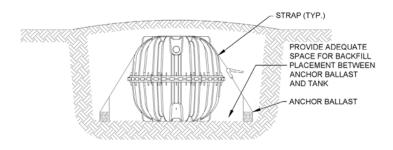
A WARNING: Use of Tank Installation Instructions: This guidance document provides general statements on backfilling and tank installation only. Refer to the Infiltrator IM- and CM-Series Tank Installation Instructions for complete tank installation requirements.
