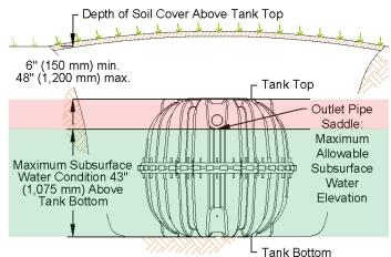
Figure 2: Buoyancy Control Parameters for Table 1
