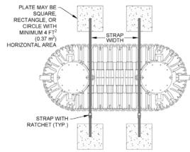
Precast concrete plate anchor ballast installation should be as follows:
