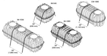
A WARNING: Do Not Use Cable Tie-Downs: The use of cables to connect anchor ballasts in lieu of strapping is prohibited. Cables concentrate the load exerted by the buoyancy control system within a small area on the tank surface, resulting in the potential to damage to the tank.
